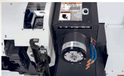
Arm type ATC + Coolant ring + LED lights
